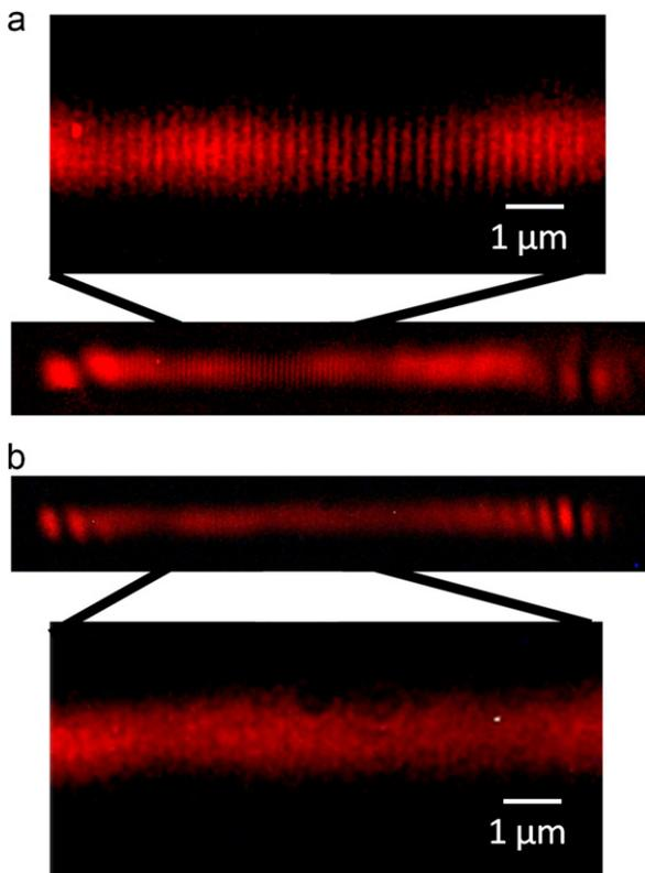
Fig. 3. SE images corresponding to two SPPs excited simultaneously in the DLSPPW. The images were obtained (a) without and (b) with a half-wave plate inserted after the high NA objective lens.
