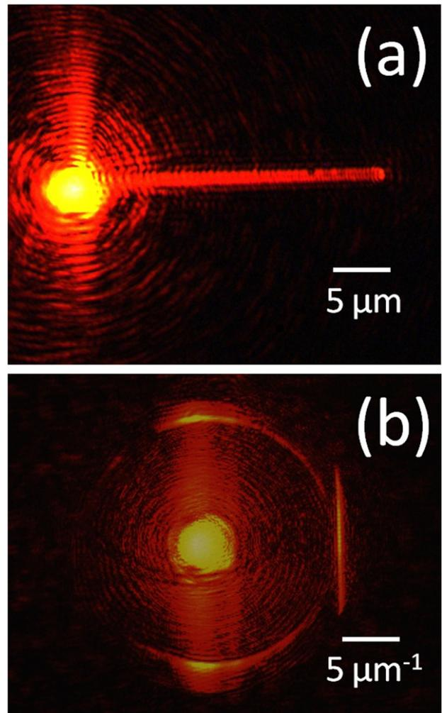
**Fig. 2.** (a) SE and (b) FP images corresponding to a single SPP excited at the left extreme of the DLSPPW. The straight vertical segment at the right extreme of the FP image is the signature of a SPP traveling from left to right in the waveguide.
