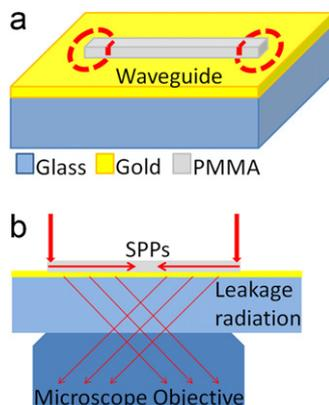
**Fig. 1.** Sketch of the (a) fabricated DLSPPW and (b) leakage radiation collection optics. The discontinuous circles illustrate the position of the laser spots used to excite SPPs by scattering at the extremes of the waveguide. The light that leaks along the paths of excited SPPs is collected by microscope's immersion oil objective lens.
